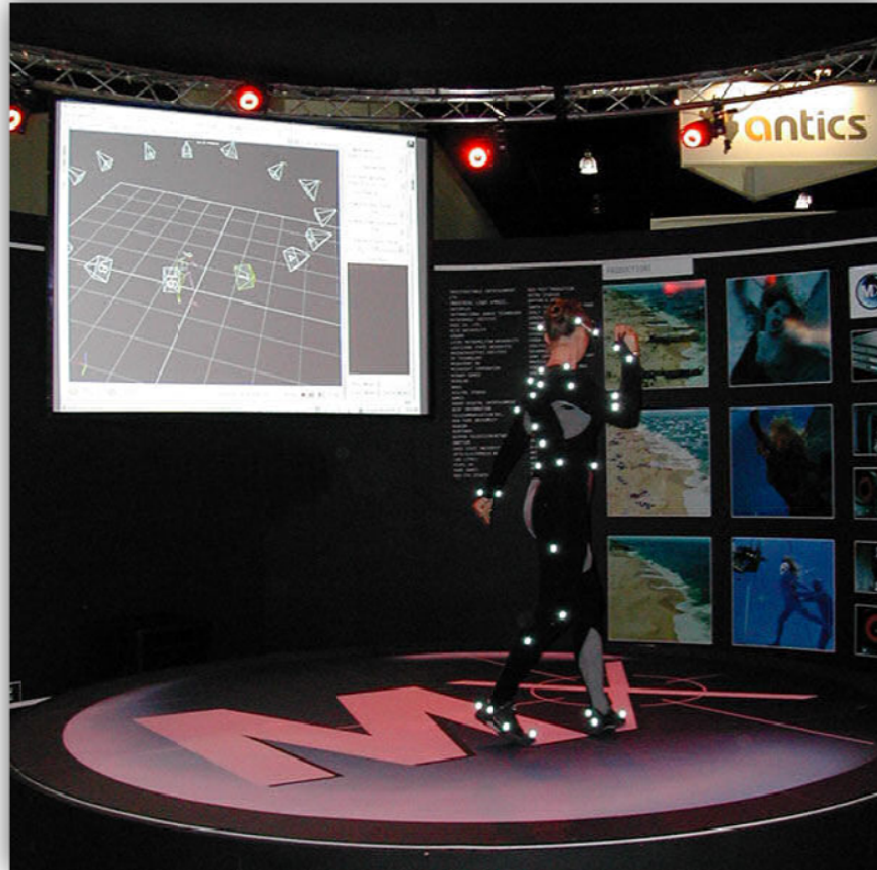
Figure 2-9: A dancer wearing a suit used in an optical motion capture system
