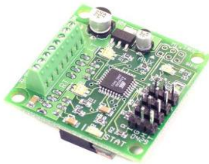
Obrázek 2.6: Scorpion Dual RC H-Bridge Motor Controller [11]
